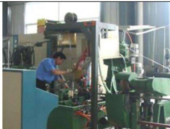
tubes (pipes) finning machines
