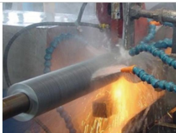
tubes (pipes) finning machines
