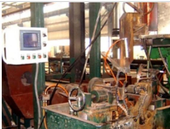
tubes (pipes) finning machines
