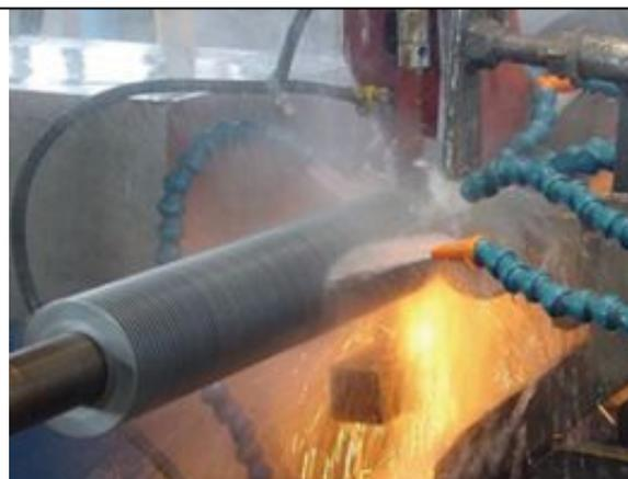
tubes (pipes) finning machines
